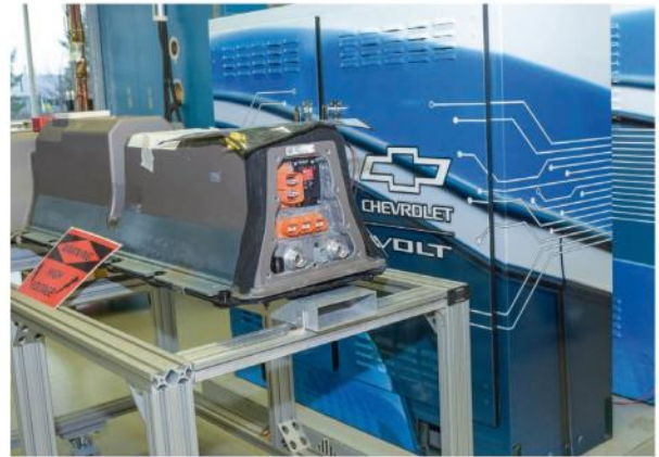
Subsequent use: In GM's battery laboratory, tests are run to see whether weakened batteries from first-generation Amperas can be used as an emergency power supply
