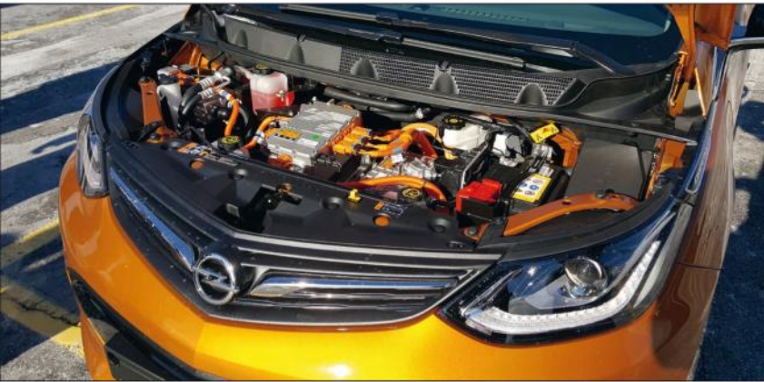
Full even without a combustor: Although the electric engine in the Ampera-e is only as large as a 5-litre beer barrel, the engine compartment is filled by power electronics, the cooler (for the battery) and the ancillary units
