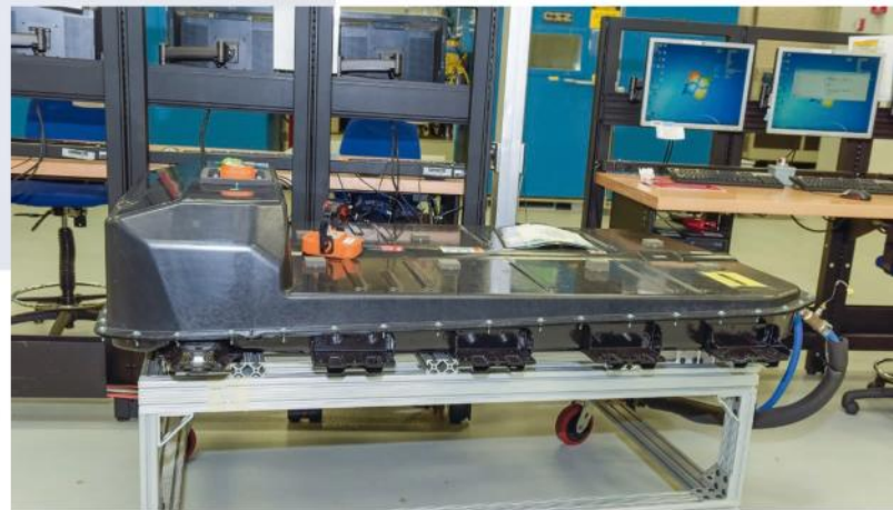
The complete battery pack weighs 430 kg. The fully-assembled pack is delivered from an LG facility in South Korea
