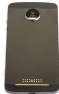
You can attach the Moto Mods to the back, and it latches on using magnets
