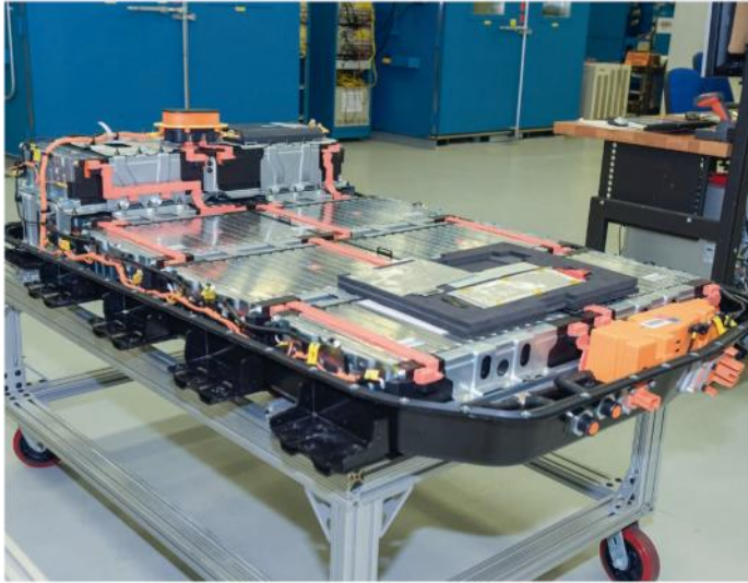
Ampera battery from within: General Motors increases the density in the battery pack by cooling from the outer sides
