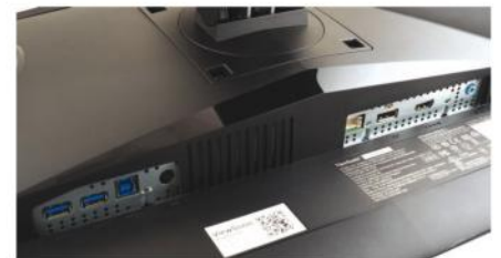
Besides the input ports, there's also two USB ports that can be enabled by connecting the USB passthrough to your PC
