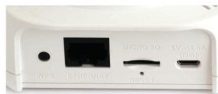
A microSD slot is located at the back. Inserting one inside allows you to use it to store recordings
